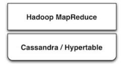
Both databases offer interfaces to the Hadoop API that allow them to act as a source and a sink for MapReduce. At a higher level, Cassandra offers integration with the Pig query language (see the Query section below), and Hypertable has been integrated with Hive.
