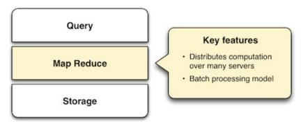
To understand how MapReduce works, look at the two phases suggested by its name. In the map phase, input data is processed, item by item, and transformed into an intermediate data set. In the reduce phase, these intermediate results are reduced to a summarized data set, which is the desired end result.
