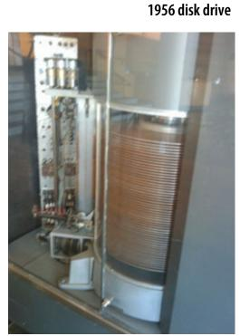
One of the first commercial disk drives from IBM. It has a 5 MB capacity and it's stored in a cabinet roughly the size of a luxury refrigerator. In contrast, a 32 GB microSD card measures around 5/8 x 3/8 inch and weighs about 0.5 gram.
