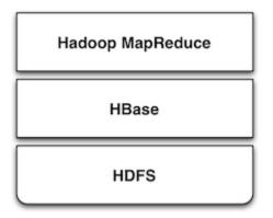
HBase uses HDFS as a storage system, and thus is capable of storing a large volume of data through fault-tolerant, distributed nodes. Like similar columnstore databases, HBase provides **REST** and **Thrift** based API access.
