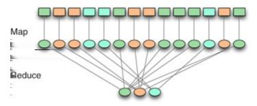
A simple example of MapReduce is the task of counting the number of unique words in a document. In the map phase, each word is identified and given the count of 1. In the reduce phase, the counts are added together for each word.
