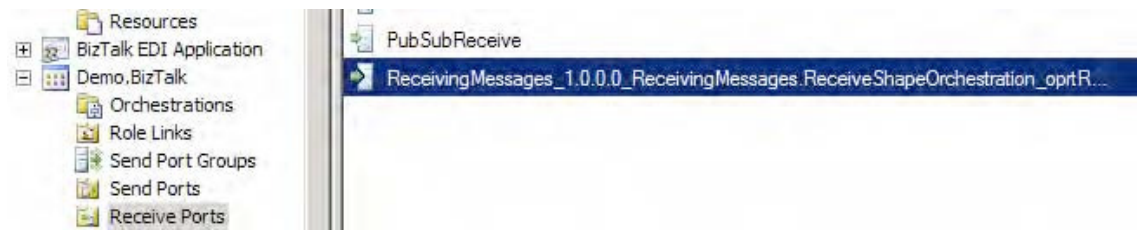
Figure 5-6. The receive port created automatically during deployment
