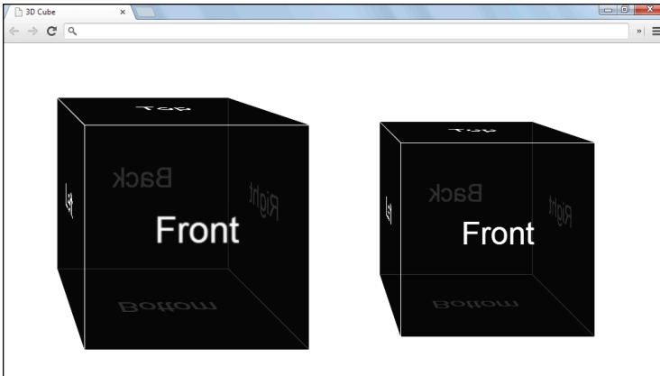
Figure 7-22 The left cube's front face is 150px closer to the viewer than it should be, causing pixelation. On the right, the whole cube element is shifted 150px further back to cancel out the original translation.
