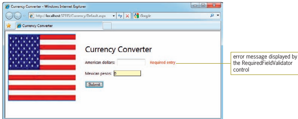
Figure 27-31 Result of clicking the Submit button when the American dollars box is empty
