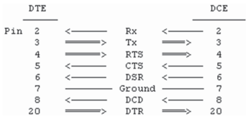
Fig. 10.8 RS232C signal lines
