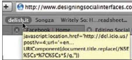
Figure 8-23. A bit o' JavaScript is all it takes to make a humble bookmark into a mighty social bookmarking bookmarklet.
