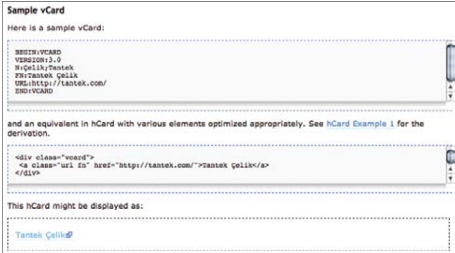
Figure 17-3. By the simple virtue of marking up your presented data with microformats, you can enable machine reading and semantic interpretation of that data by third-party developers.
