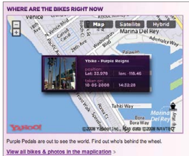
Figure 5-21. The Purple Pedals GPS-Flickr Bikes automatically take pictures, tag them with geolocation, and upload them to Flickr (much like the Blogging in Motion purse).
