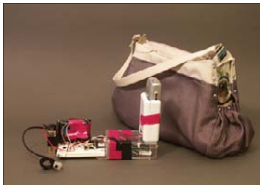
Figure 5-20. The Blogging in Motion hack combines a camera phone, a purse, a pedometer, a GPS parser called ZoneTag, and a Flickr account to enable automated regular live photoblogging of the life of the person carrying the purse.
