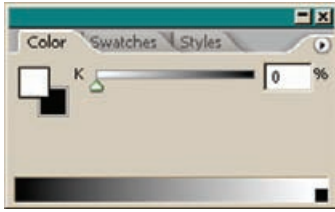
FIGURE 3-10 The Grayscale color slider in Adobe Photoshop provides access to a range of 256 different gray values.
