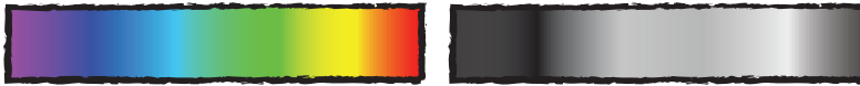
FIGURE 5-4: The rainbow color scale (left) does not consistently increase in brightness, as shown in the grayscale image of the same rainbow color scale (right). Do not use a rainbow color scale for magnitude.
