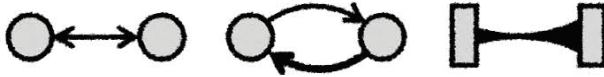
FIGURE 4-19: This shows bidirectional flows with overlapping links, curved links, and a chord link.
