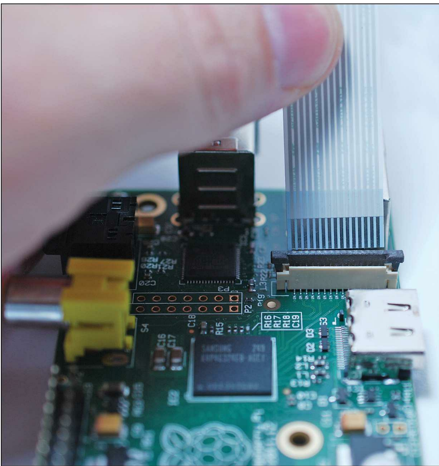
FIGURE 16.4 The Camera Board installation procedure is a bit tedious, and the components are certainly delicate.
