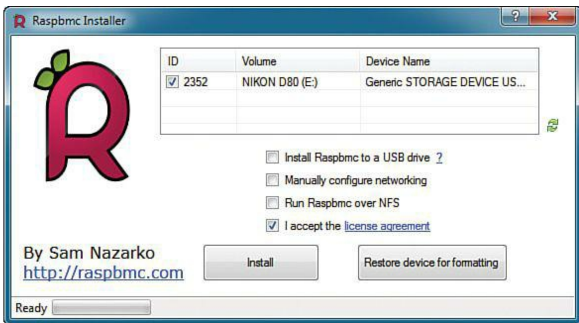
FIGURE 12.2 You can flash your SD card under Windows by using the Raspbmc Installer application.
