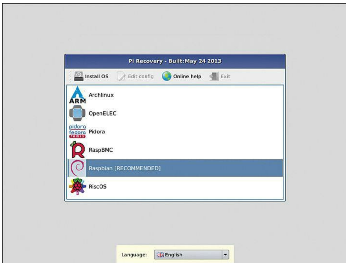
FIGURE 4.11 The NOOBS utility makes it much easier to load an OS on your Raspberry Pi.
