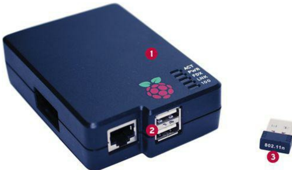
FIGURE 7.2 Adafruit sells very reasonably priced USB Wi-Fi dongles. Regarding the annotations: 1 shows the Raspberry Pi in a nice case; 2 shows the two USB ports on the Model B board; 3 shows my Adafruit Wi-Fi dongle.
