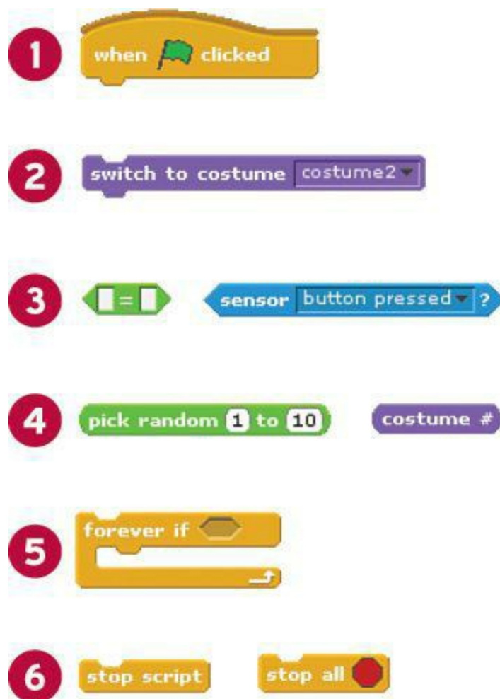
FIGURE 8.5 A mash-up showing you the different types of block shapes in Scratch. Here's a key to the annotations: 1: Hat block; 2: Stack block; 3: Boolean block; 4: Reporter block; 5: C block; 6: Cap block.
