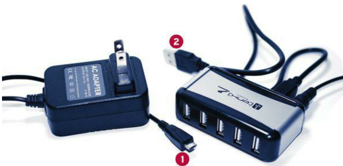
FIGURE 2.3 A Raspberry Pi-compatible power supply on the left (Micro USB plug is labeled 1) and a powered USB hub on the right (Standard USB plug is labeled 2).
