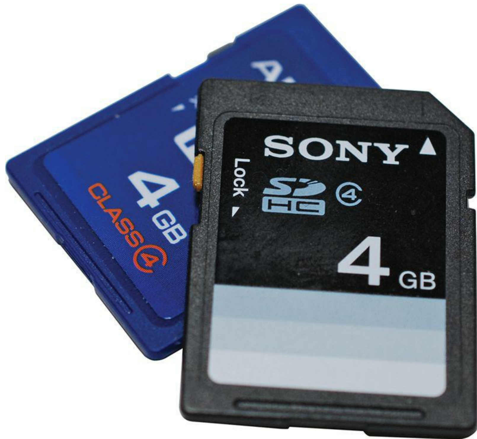
FIGURE 4.5 You can learn much about an SD card by studying its sticker label. Here we can see the brand, capacity, and speed rating in a single glance.
