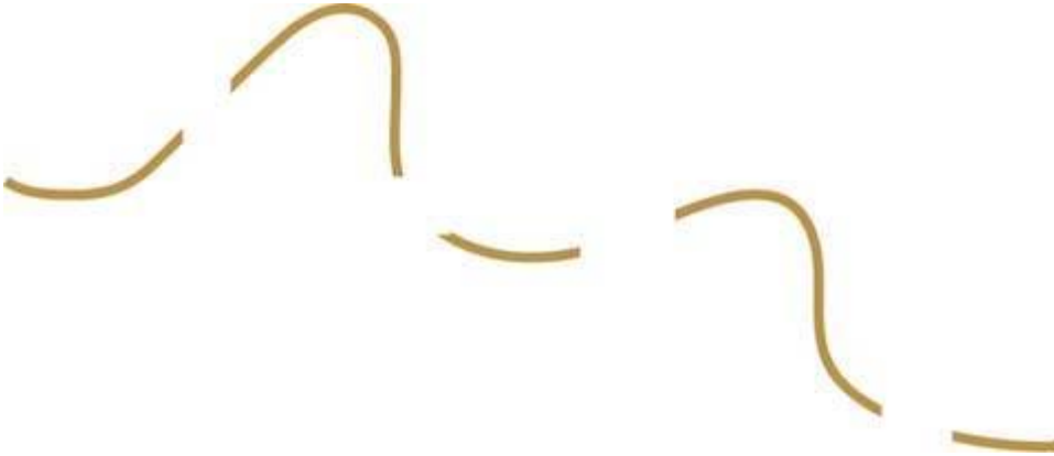
Figure 4-16. The Gestalt principle of continuity explains why we see this as a single wavy line.
