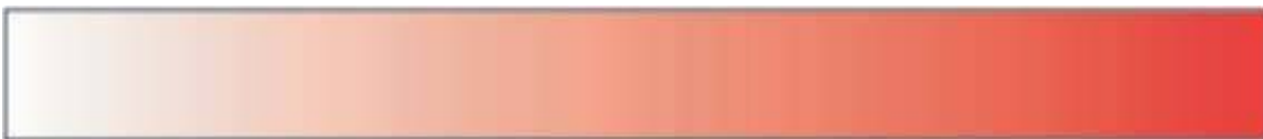
Figure 4-3. The full range of color saturation, in this case of the hue red, with 0% saturation on the left and 100% saturation on the right.
