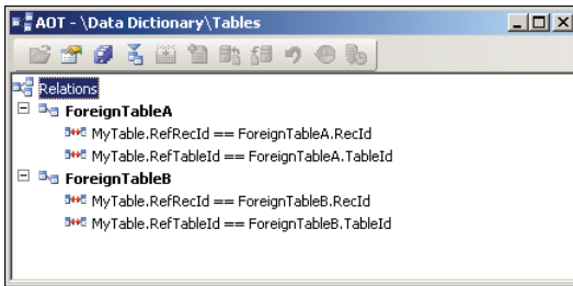
FIGURE 4-4 An association to any record in a fixed set of tables.
