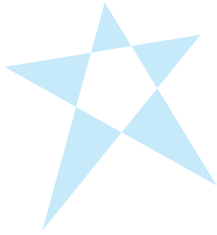
FIGURE 6.34 Filling with the odd-even test.
