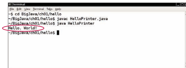
Figure 6 Running the HelloPrinter Program in a Console Window
