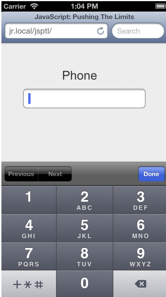
Figure 5-7 This numeric keypad displays in iOS for <input type="tel"> .
