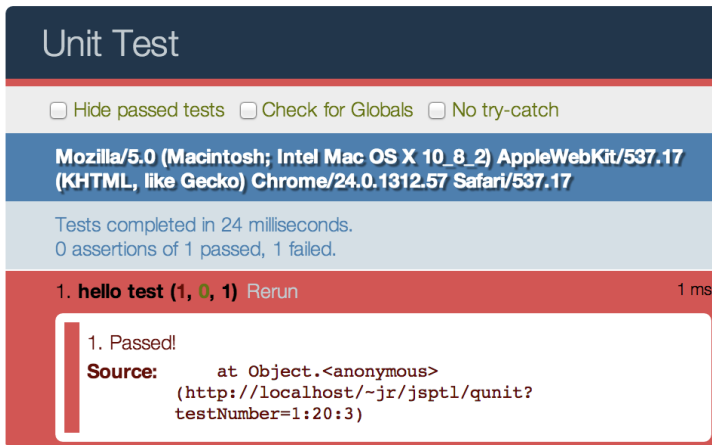
Figure 1-13 When the unit test fails, QUnit outputs a fail message and the source of the error.
