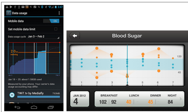
FIGURE 6-38. Data Usage for Android and Diabetes concept app by Anthony Lagoon: Threshold line and band, respectively
