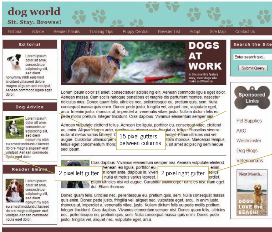
Figure 12-8 Gutter measurements in the layout
