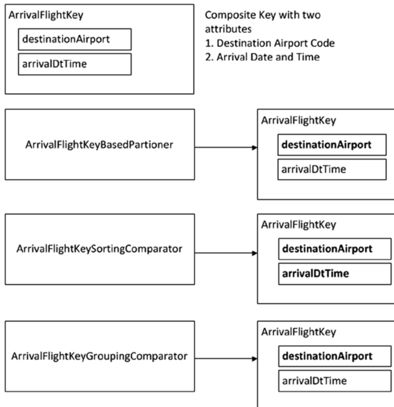
Figure 6-3. Components for Secondary Sort and how they use the key attributes
