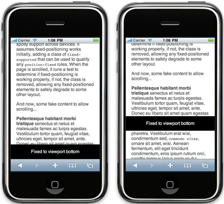
FIG 2.17: Intended behavior (left) vs. buggy behavior (right) in a browser with poor fixed-position support.
