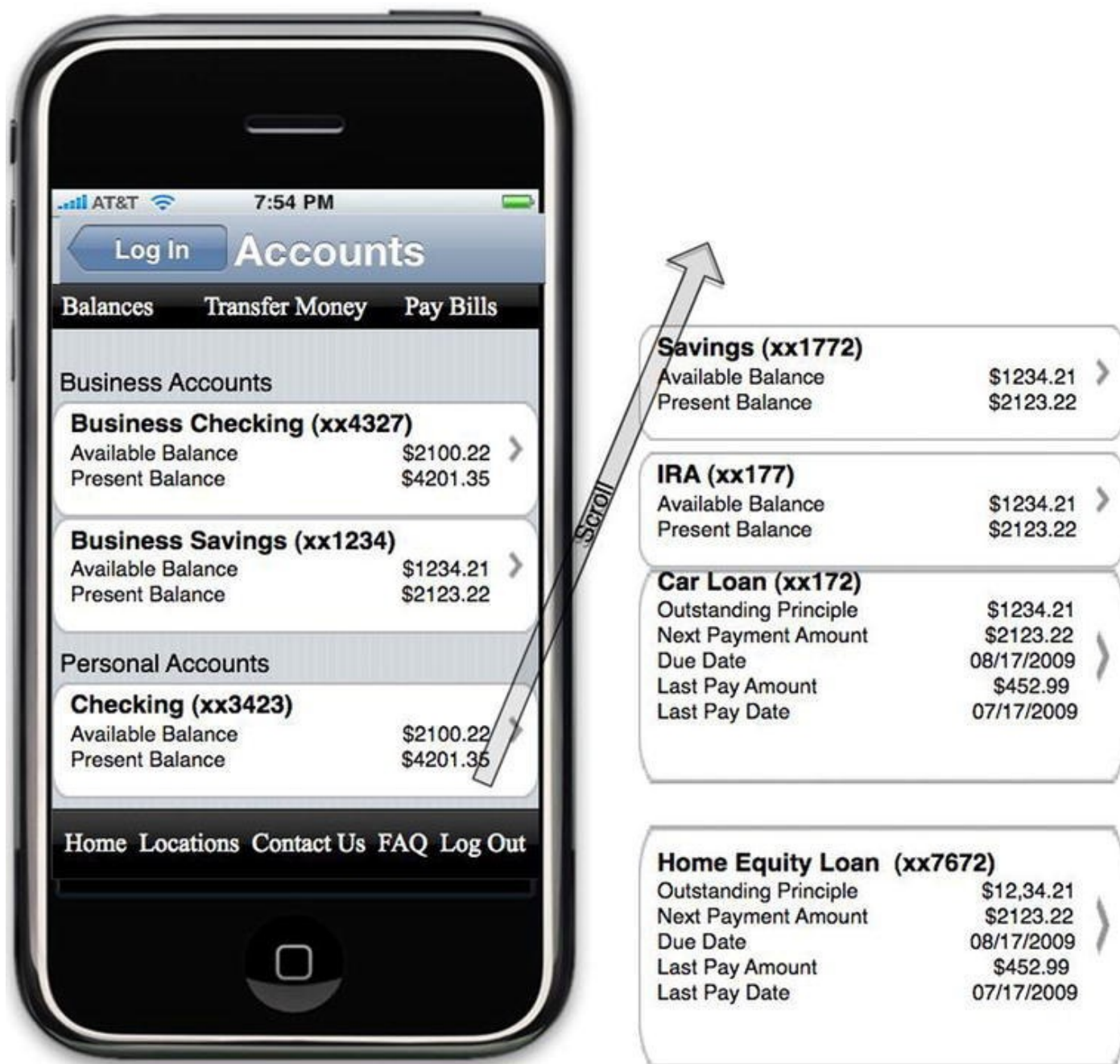
Figure 1-1. This is a UI mock-up of the account balance screen for an iPhone mobile banking app before development begins on the original iPhone in 2010. This UI design mock-up was completed using OmniGraffle
