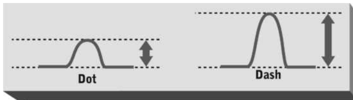
FIGURE 8.5 Wave amplitude representing Morse code dots and dashes Courtesy of Course Technology/Cengage Learning
