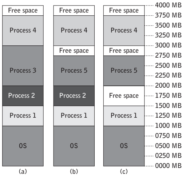
FIGURE 11.16 Changes in memory allocation as processes execute and terminate Courtesy of Course Technology/Cengage Learning
