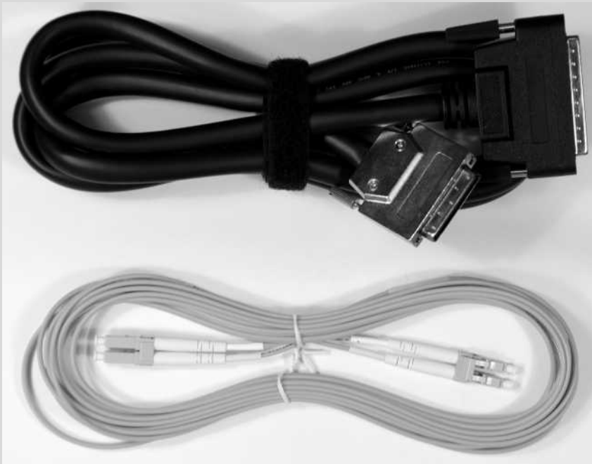
FIGURE 8.26 Parallel SCSI-3 (top) and serial optical (bottom) cables Courtesy of Course Technology/Cengage Learning
