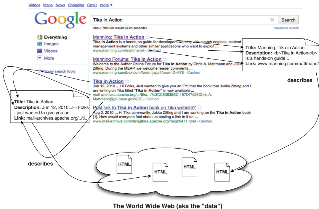
Figure 6.1 The search engine process and metadata. Metadata about a page, including its title, a short description, and its link are used to determine whether to “click” the link and obtain the content.
