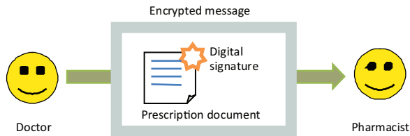
Figure 11.1 Illustration of how a digital prescription document can be used to securely transfer accurate prescription information from a doctor to a pharmacy. A digital signature ensures that the document came from someone authorized to make prescriptions, and encryption is used to ensure the privacy of the patient.
