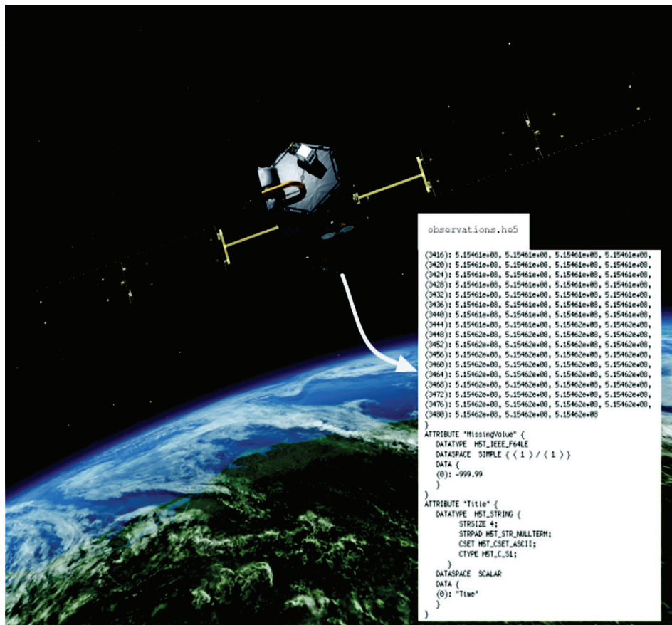
Figure 8.2 A postulated satellite scenario, observing the earth and collecting those observations in data files represented in the Hierarchical Data Format (HDF). HDF stores data in a binary format, arranged as a set of named scalars, vectors, and matrices corresponding to observations over some space/time grid.
