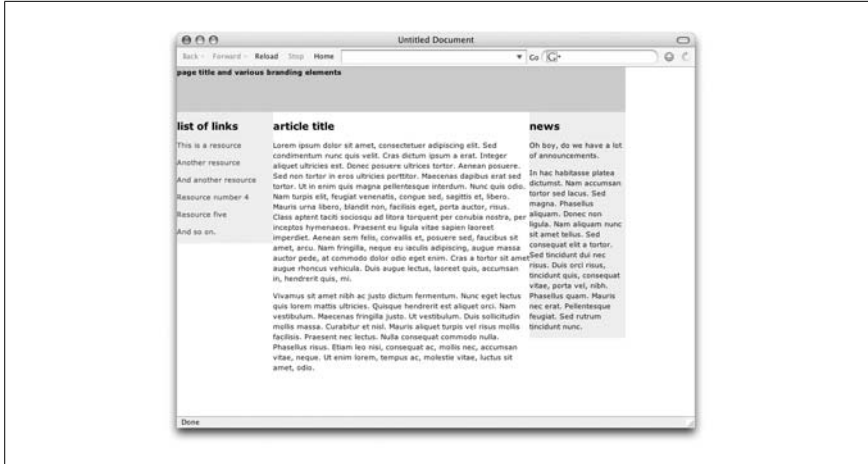
Figure 24-6. Absolutely positioning all three columns
