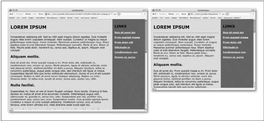
Figure 3-4. A web page with a liquid left column and a fixed-width right column
