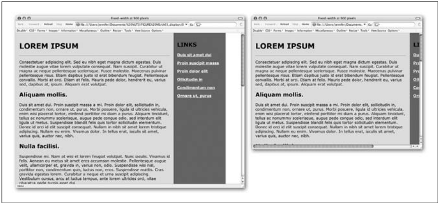
Figure 3-2. A fixed-width web page with exact pixel measurements viewed on large (left) and small (right) monitors
