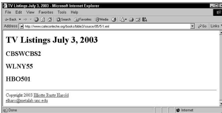
Figure 5-5: The station networks, call letters, and channels displayed as H2 headers when the XSLT style sheet in Listing 5-5 is applied
