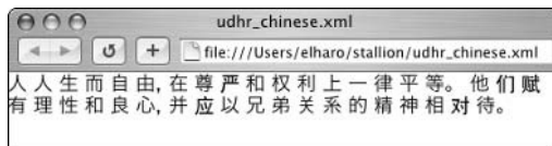
Figure 6-2: Browsers convert numeric character references into the actual characters before displaying them.
