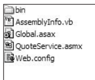
Figure 30-1: Files and directory needed for a release version of a .NET Web Service
