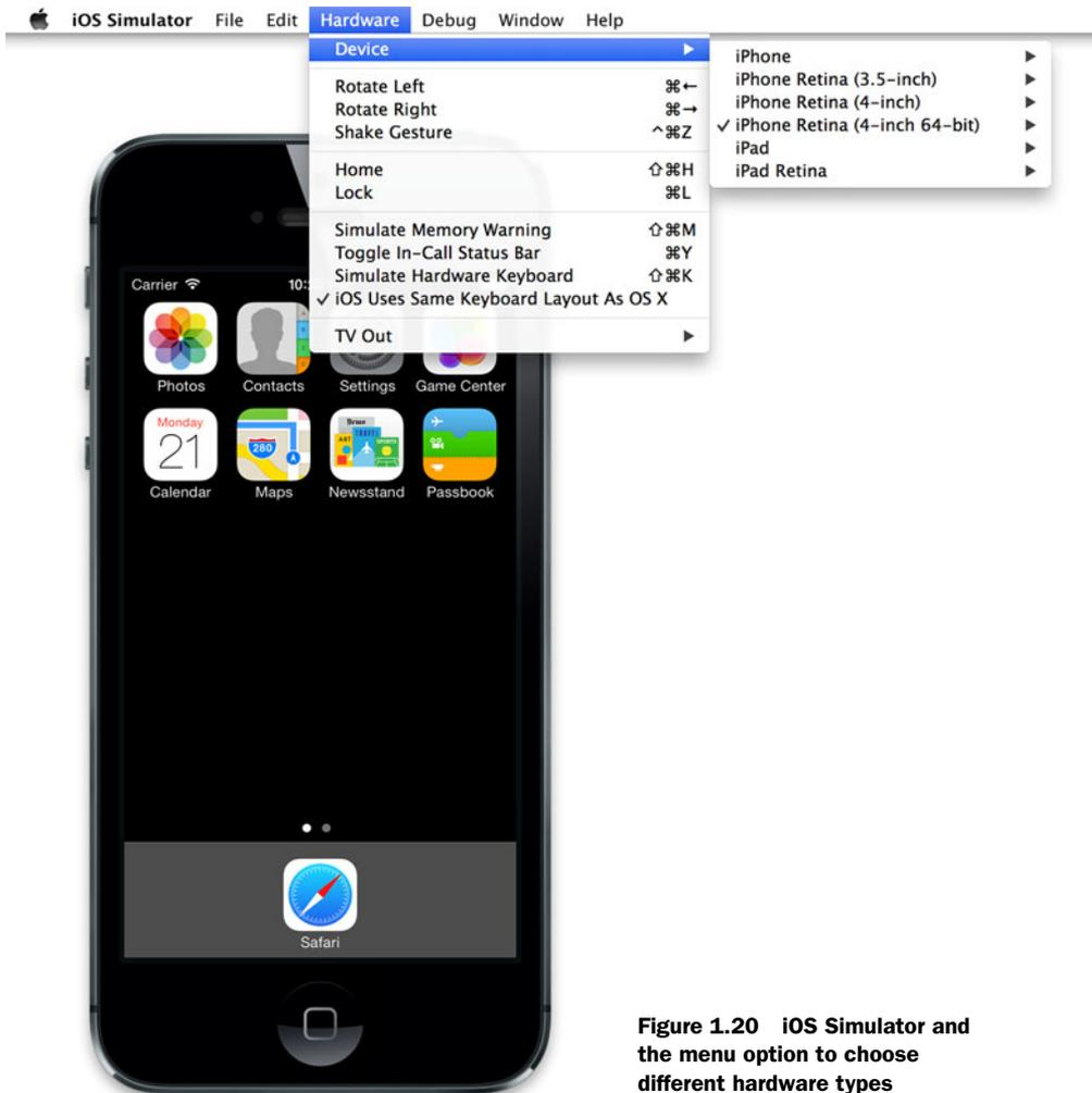
**Figure 1.20** iOS Simulator and the menu option to choose different hardware types
