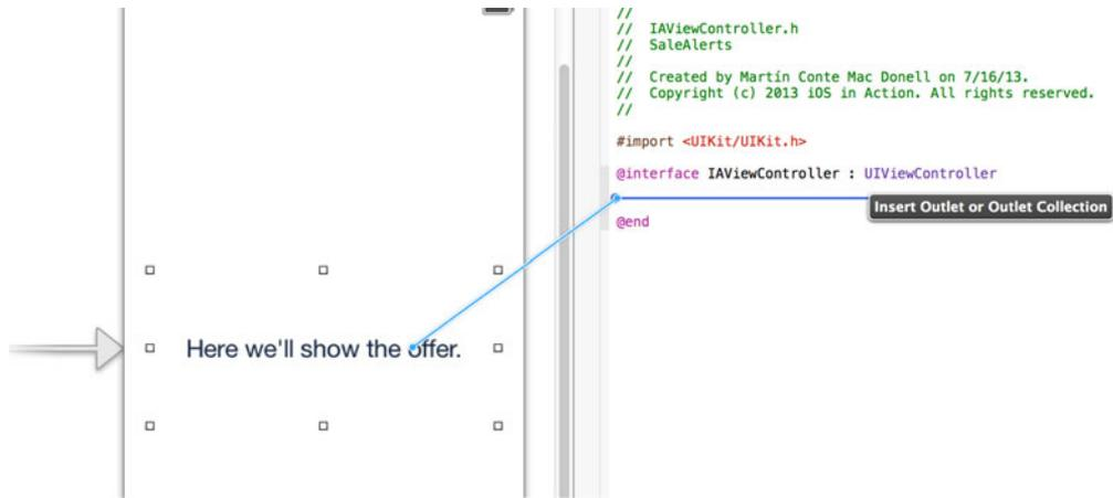
**Figure 13.12** Linking the offer label to the `IViewController` public definition
